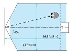
Use the optional external 3D emitter if you cannot view the 3D image normally or if the projector is located more than 16.5 feet (5 m) from the viewing area. See "Optional Accessories" on page 9 for ordering information.
